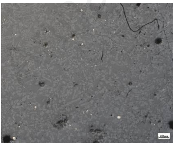
Figure 44. Olivine crystals (light grey), copper matte (yellow), glassy matrix (dark grey) (RL).
