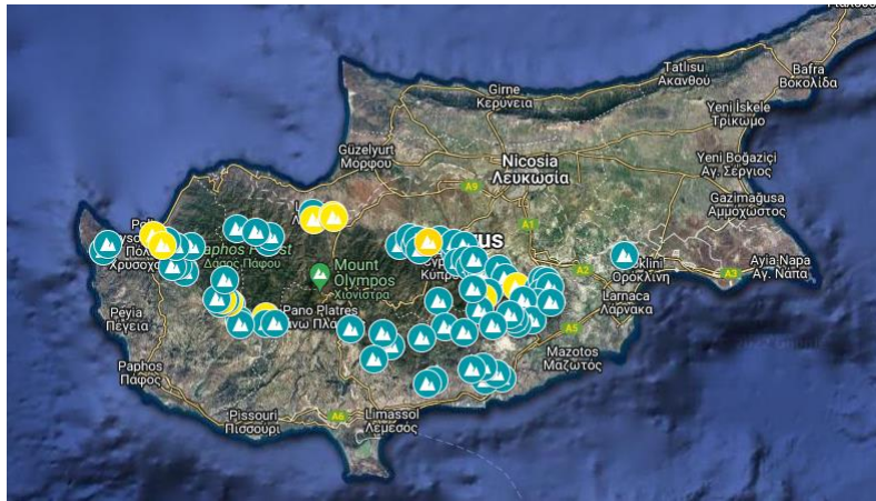
Figure 7: The map of Cyprus, with blue are the recorded slag heaps of the island and with yellow the ones that analysis showed that are manganese rich.
