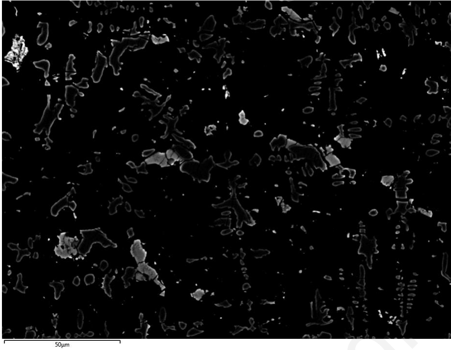
Figure 111. Sample PEL38. When the photo was taken in the SEM-EDS, a high contrast was applied, with little brightness. The formations shown are copper matte (bright grey) which is very closely associated with free iron oxides (only their outline is visible).
