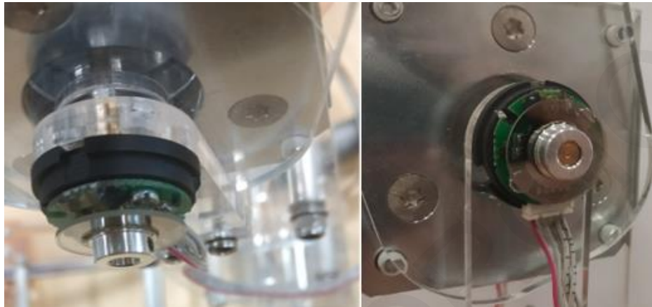
Figure 22: Optical Encoder installation.
