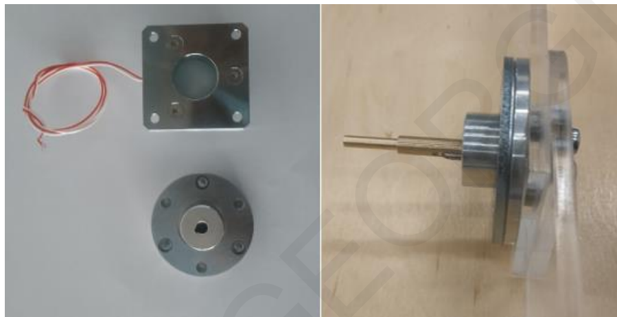
Figure 12: Electromagnetic break assembly,
