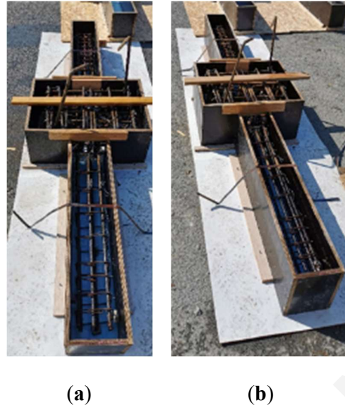
Figure 5. 4: Specimens' molds and steel reinforcement configuration: (a) with continuous longitudinal bars; (b) with lap-spliced bars.
