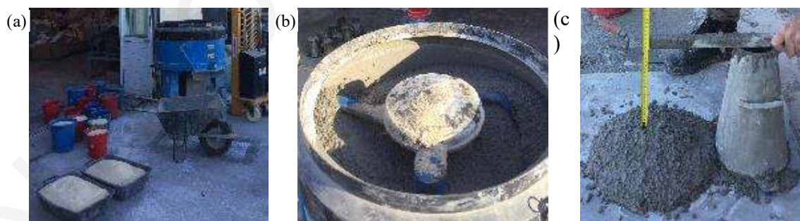
Figure 4. 6: (a) Dry Aggregates; (b) Mixing after water addition; (c) Concrete slump test
