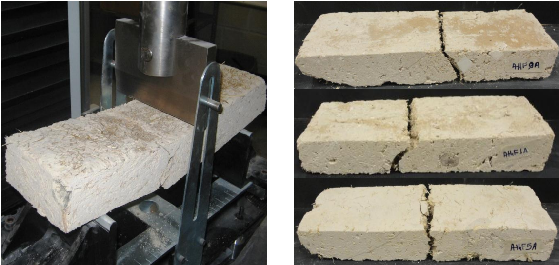
Figure 3.13: Flexural failure of half brick adobe specimens. Note that in certain cases failure did not occur in the middle of the sample, as expected; instead it propagated through pre-existing planes of weakness, such as shrinkage cracks and areas where stones or gravel disrupted the homogeneity of the soil matrix.
