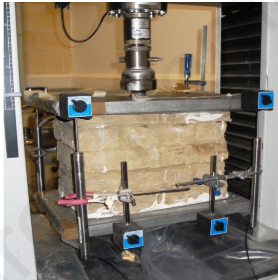
Figure 4.5: Experimental set-up used for the implementation of displacement-controlled loading-unloading compression tests on running bond adobe wallettes.
