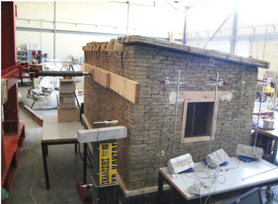
Figure 6.3: Test set-up used for the implementation of monotonic lateral loading on a 1:2 scaled adobe masonry building.
