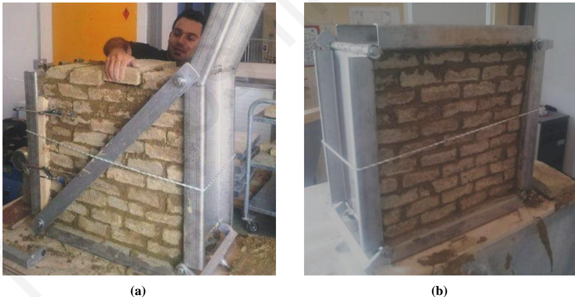
Figure 4.13: The adobe masonry wall specimen used in the diagonal tension tests (a) during and (b) after its construction.
