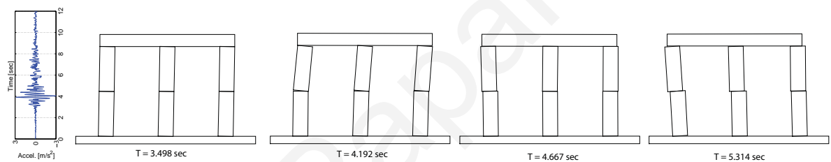
Figure 7.1. Time-history response of a colonnade with two drums under an accelerogram from the Athens Earthquake scaled to a PGA of 32.21 \text{ m/sec}^2 .
