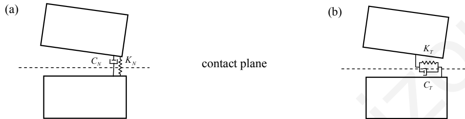
Figure 3.2. Contact springs and dashpots: (a) in the normal and (b) tangential directions.
