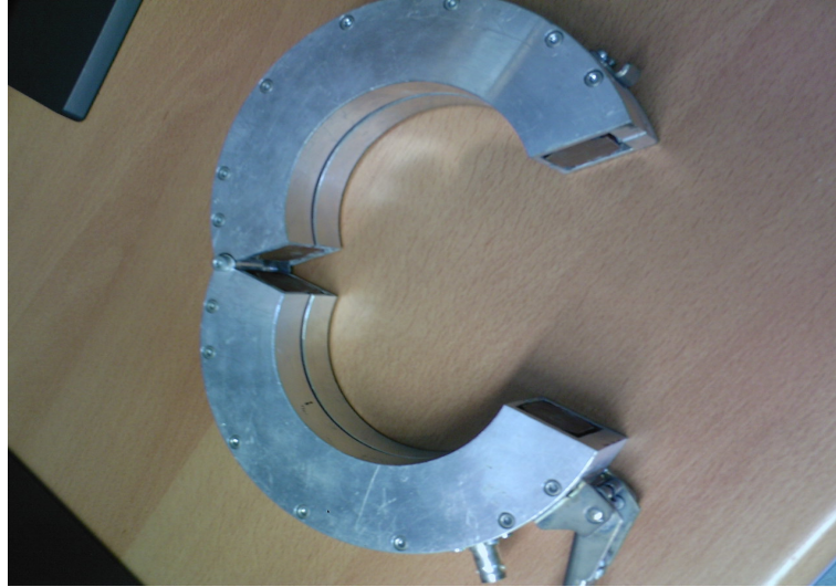
Figure 2.5: Commercial HFCT (IPEC 140/100) analysed
