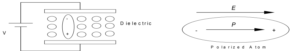
(a) Parallel plate capacitor with dielectric material inserted between the conducting plates. (b) Dipole moment p in each molecule.
