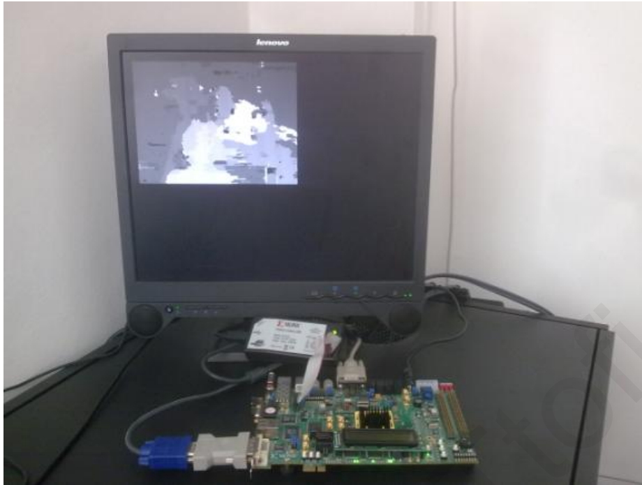
Figure 3.6: FPGA implementation used to verify the proposed architecture.
