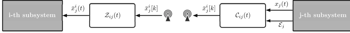
Figure 6.1: Block diagram of the broadcast of x_j to the i -th subsystem.
