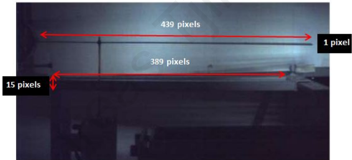
Figure 35: Pixels to mm conversion using cantilever beam and object of known dimensions
