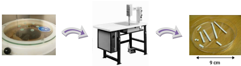
Figure 3.10 Schematic drawing of PVC nanocomposites fabrication with Branson ultrasonic welder
