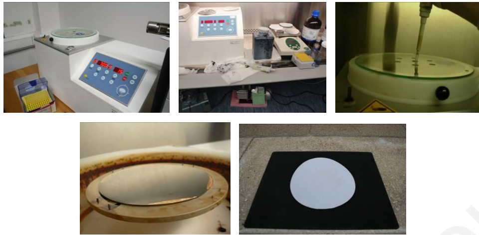
Figure 3.7 Dispersion of different nanofluids onto the PVC foils using a Delta6RC TT spin coater device
