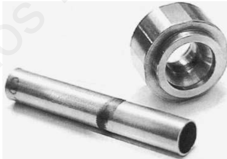
Figure 6: Wear specimen (ring and tube), both in 304L stainless steel. Figure taken from [40] .
