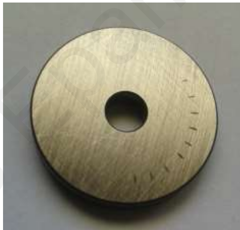
Figure 71: The circular crater pattern on the hardened stainless steel (1.4031/X38Cr13) sample tested in Mode 3.
