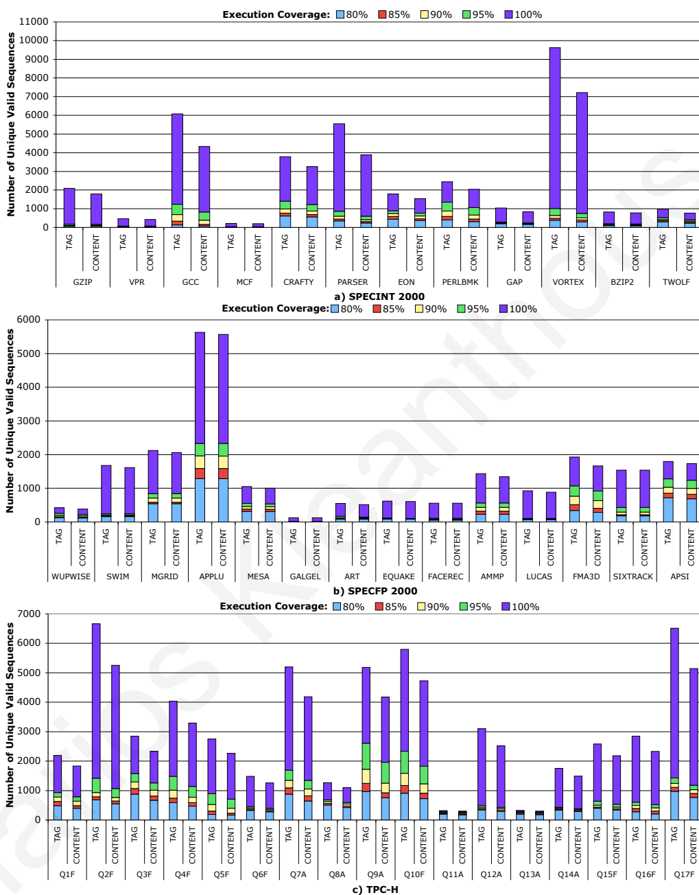
Figure 6: Execution coverage of unique valid blocks for the a) SPECINT 2000, b) SPECFP 2000 and c) TPC-H benchmarks
