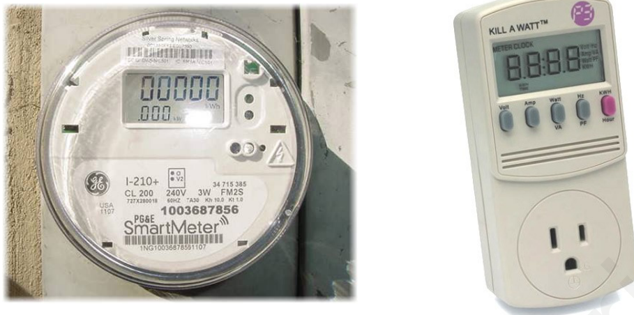
Figure 2.2: A typical residential smart meter (left) and a smart power outlet (right).
