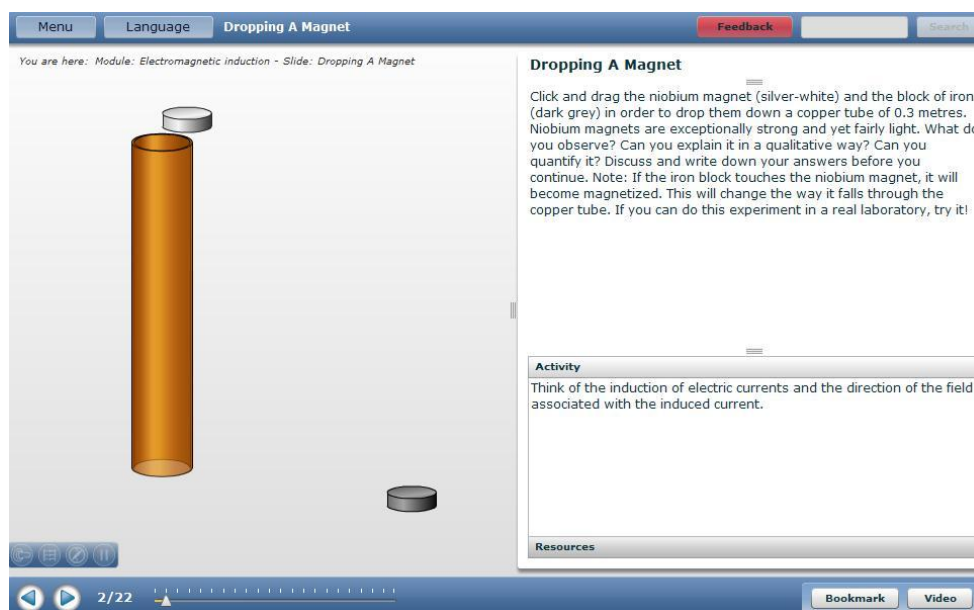
Figure 1. Screen shot from on-line modules application showing the animation of a magnet falling down the copper tube
