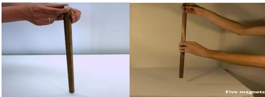
Figure 3. Real time experiment with magnet falling through copper tube
