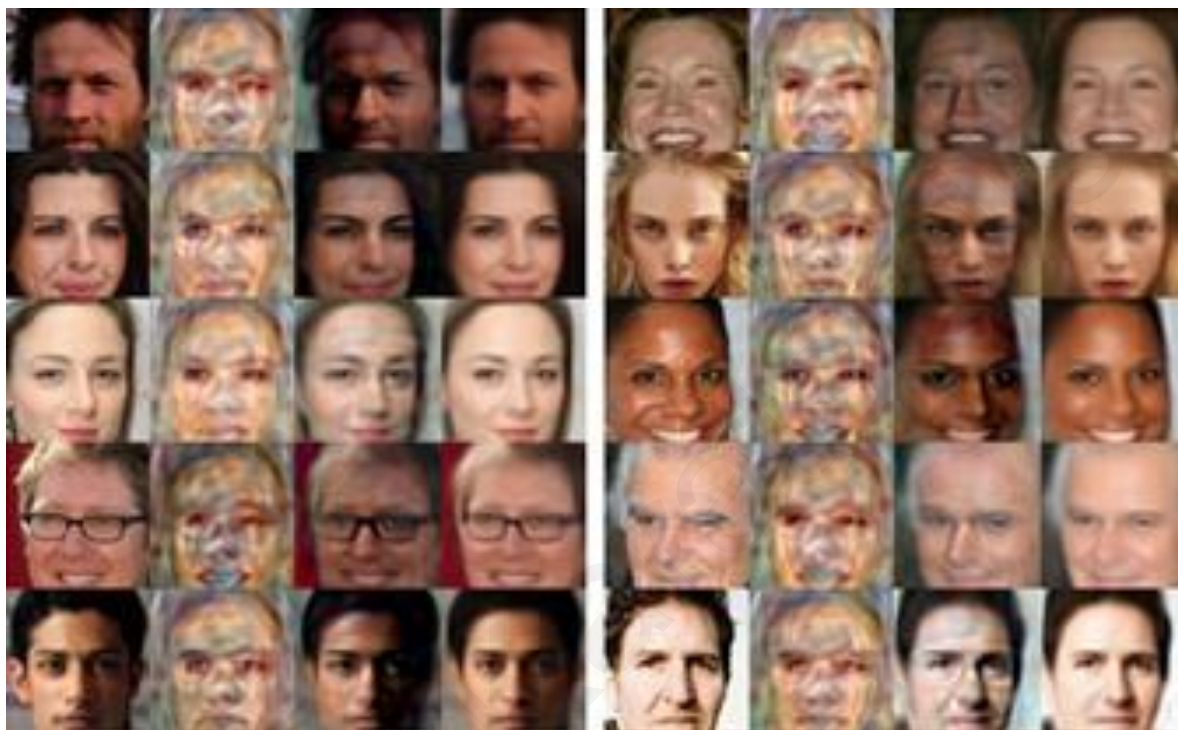
Figure 5.14: The output of the model after masking out (omitting) either the contribution of the classifier (3 rd column) or the contribution of the encoder (2 nd column). The normal output without any masking is shown in the 4 th column.
