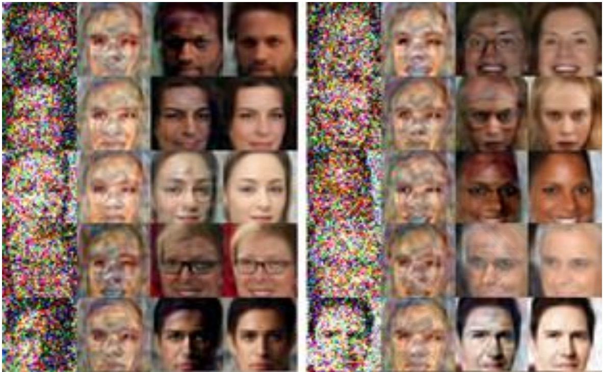
Figure 5.15: The output of the model when the input is corrupted with Gaussian noise (1 st column) and either the contribution of the classifier is masked (3 rd column) or the contribution of the encoder is masked (2 nd column). The normal output without any masking is shown in the fourth column.
