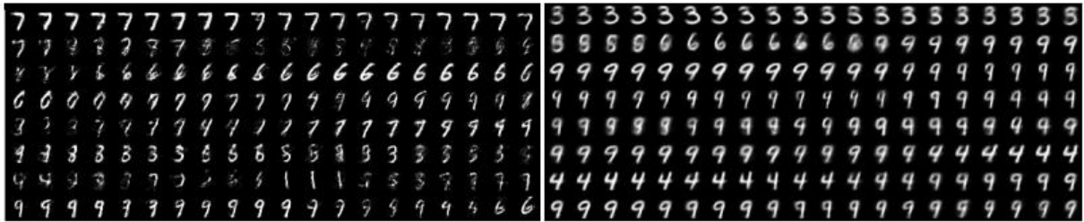
Figure 4.3: Samples drawn from a denoising autoencoder trained on MNIST digits. On the left, the samples of a model not implementing the walk back procedure are shown. On the right the samples drawn from a model implementing the walk back procedure suggest that there are less spurious samples [122].
