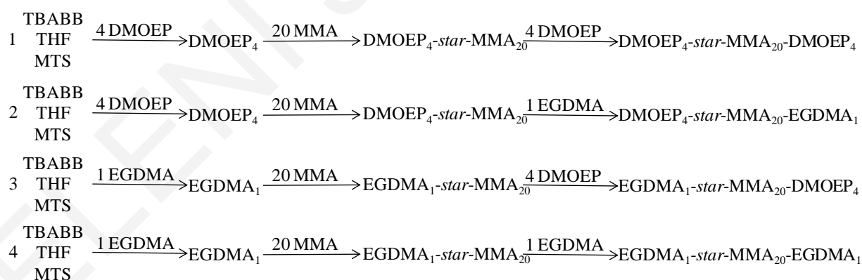
Figure 2.1. Synthetic sequences followed for the preparation of the end-linked MMA homopolymer networks based on interconnected “core-first” star polymers.
