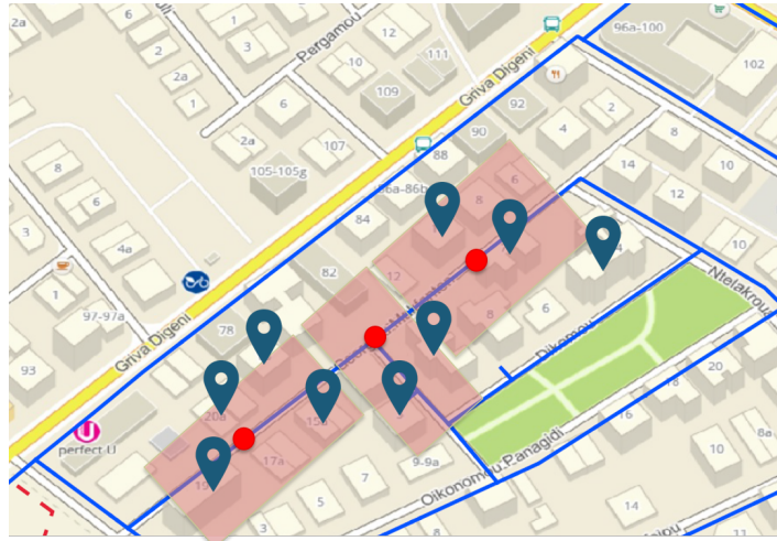
Figure 1.3. Grouping of consumers into nodes in a GIS using building open data.
