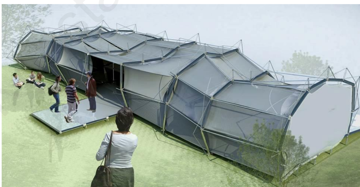
Figure 1.2: The concept of a reconfigurable building, as a variable geometry structure (Matheou et al. 2013)
