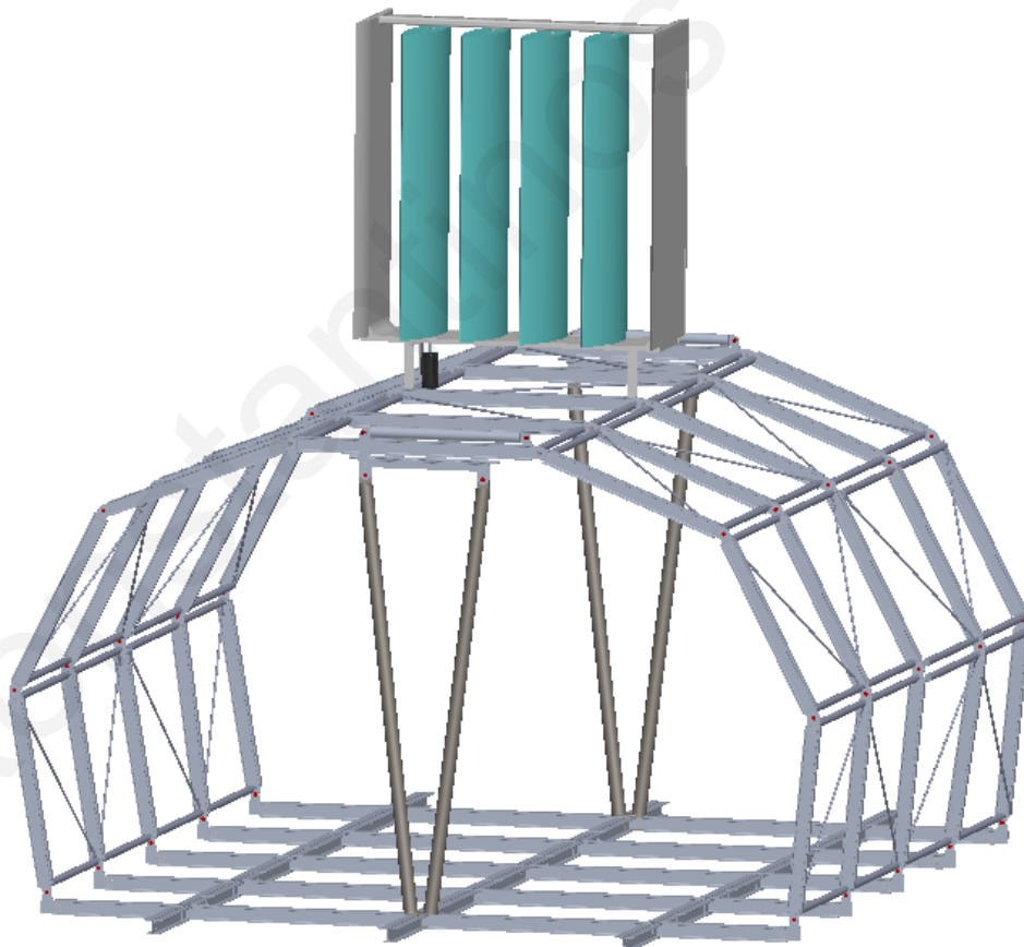
Figure 6. 8: Aerodynamic system assembled in the construction (conceptual design)
