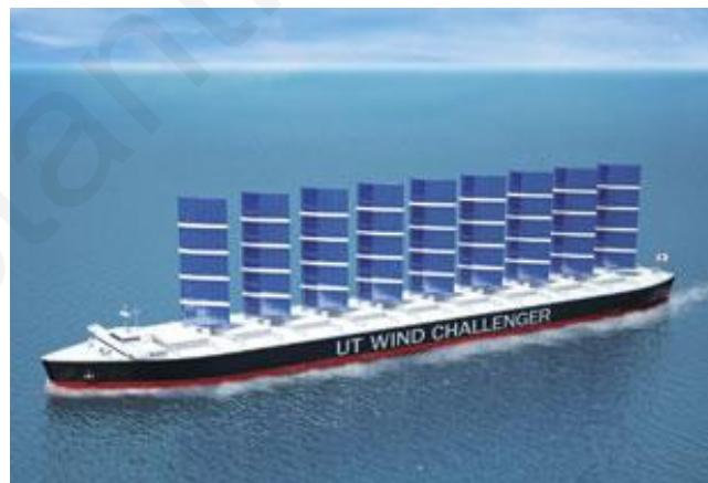
Figure 6.2: Wind-assisted shipping (Seaspout 2012)
