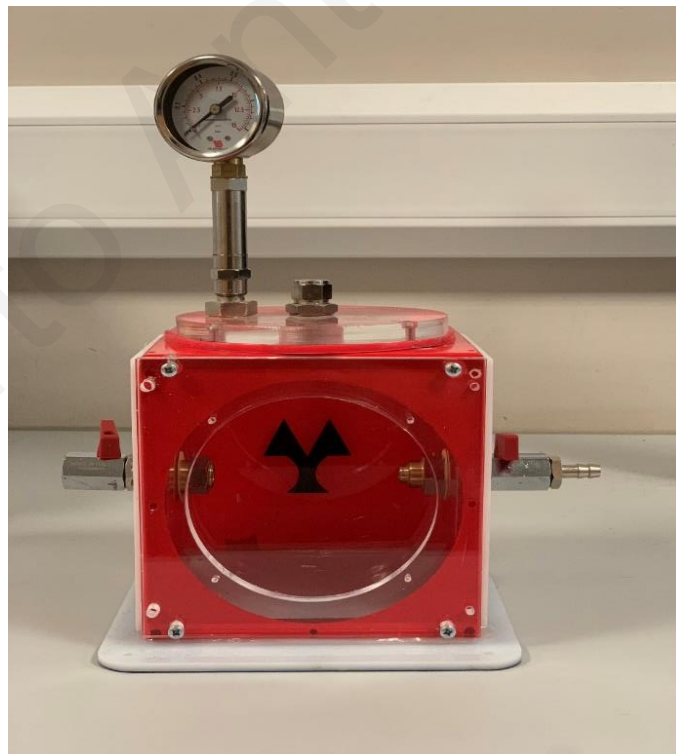
Figure 23: Schematic set up of the chamber that will be used in the performance of gas sensing experiments for ammonia detection and photograph of the actual chamber that was manufactured
