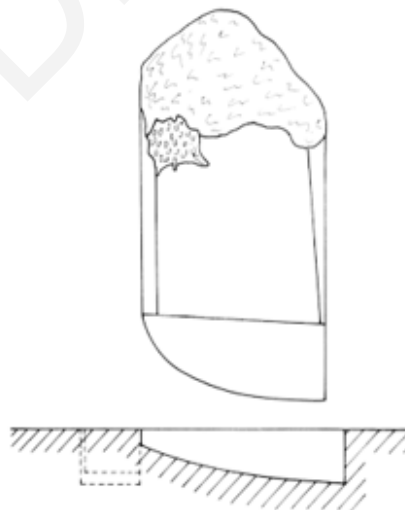
Figure 55: The mast base and the main cavity of the Dramont E mast-step (Santamaria 1984: 109, fig. 3).
