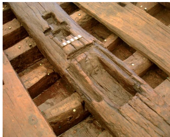
Figure 34: The notches on the upper face of the Napoli A keelson/ mast-step (Boetto & Poveda 2018: 35, fig. 26).
