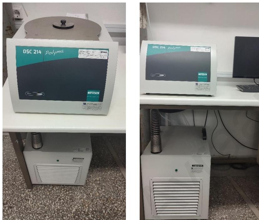
Figure 2.15: Differential Scanning Calorimeter (DSC 214 Polyma, Netzsch) which is located in the Advanced Materials & Devices Laboratory at Aristotle University of Thessaloniki
