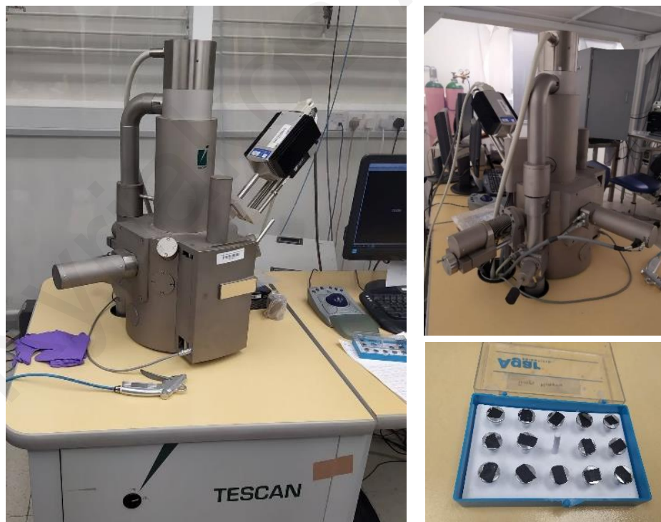
Figure 2.14: Scanning electron microscopy (Vega TS5136LS- Tescan) which is located in the Department of Mechanical and Manufacturing Engineering at the University of Cyprus.
