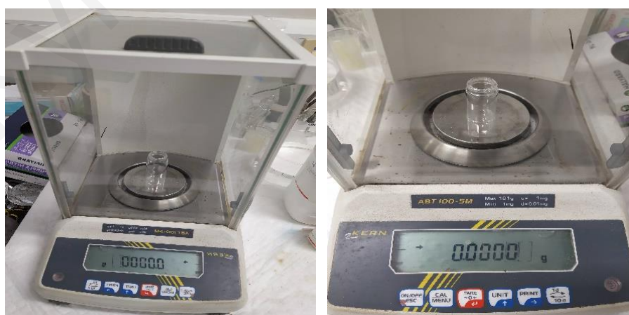
Figure 2.4: The vials were placed on the high precision weighing scale followed by the reset of the weighing scale
