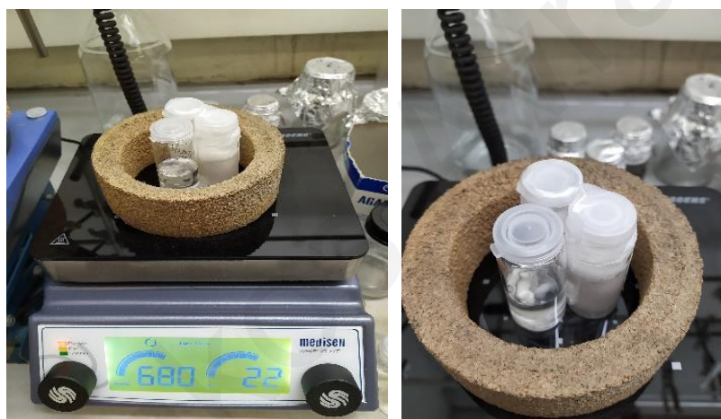
Figure 2.9: Magnetic stirring of the prepared solution for a day at 680 rpm under ambient conditions
