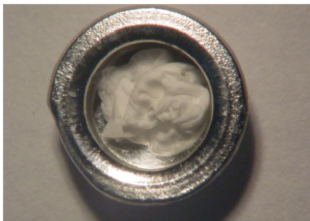
Figure 3.29: PEO/ PMMA (80/20)/ 10% n-eicosane after 30 thermal cycles (until 48°C)
