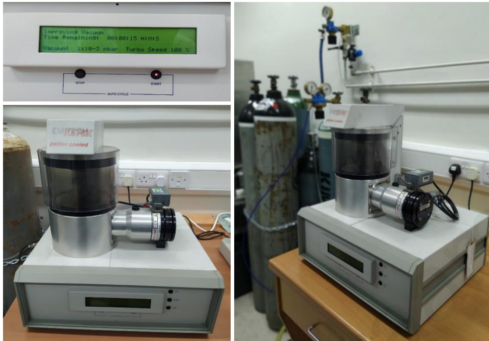
Figure 3.13 Sputtering system (K575X Turbo Sputter Coated- Emitech, Bal- tec SCD 500) which is located in the Department of Mechanical and Manufacturing Engineering at the University of Cyprus.
