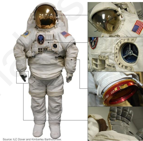
Figure 1.11 Space suits and gloves using phase change materials [31]
