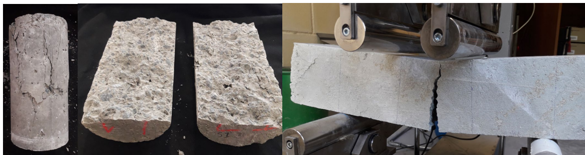
Figure 6: Top: Compressive stress-axial strain-lateral strain of LSC specimens. Bottom: Failure patterns under uniaxial compression (left), split cylinder (middle) and four-point bending (right) tests.
