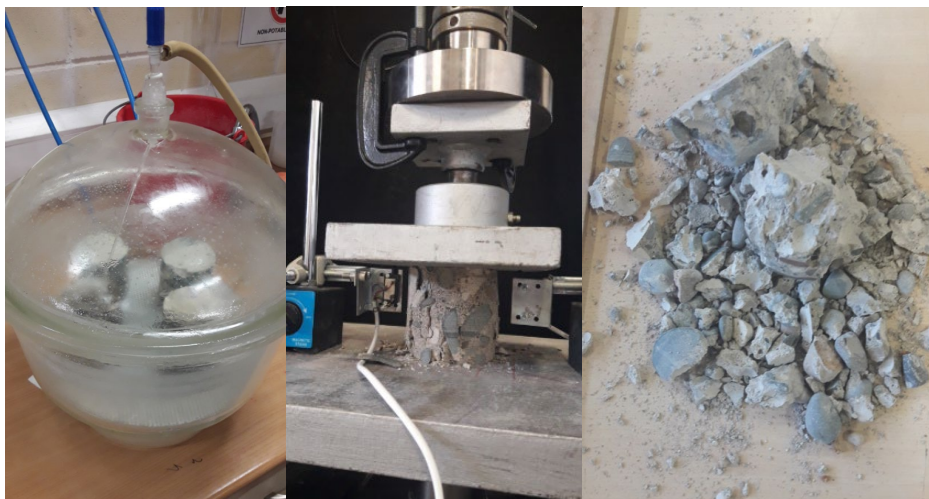
Figure 4: Tests on concrete. Left: Specimens for porosity measurement in the vacuum vessel. Middle: Testing apparatus for concrete compression. Right: Failure of concrete specimen in compression.
