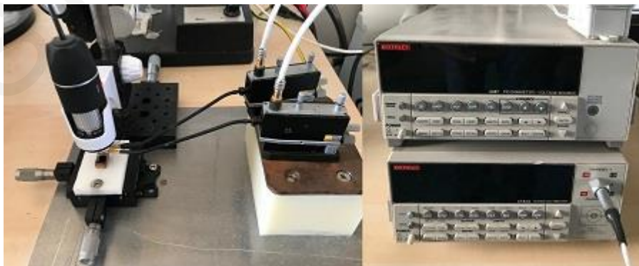
Figure 3.11 Dark IV setup with two-probe configuration.
