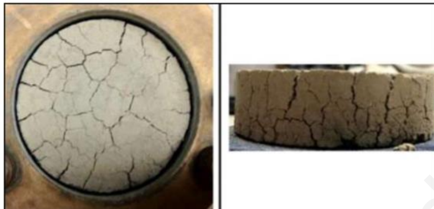
Figure 12 - Top view (left) and side view (right) of a soil sample after shrinkage (from Firoozi et al. (2016))
