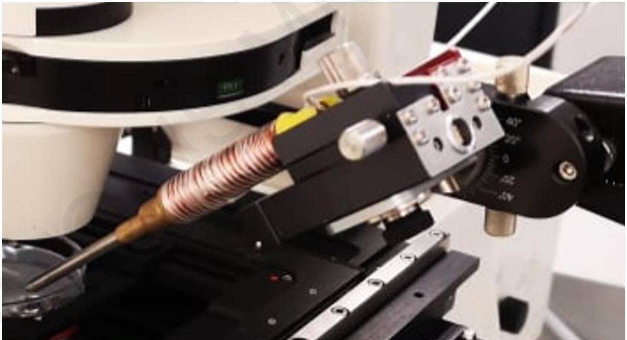
Figure 12: Close up of the magnetic tweezer that shows the brass frame with the windings creating a solenoid. One end of the metal core is attached to micromanipulator and the tapered tip is inserted into glass coverslip in a 45-degree angle.
