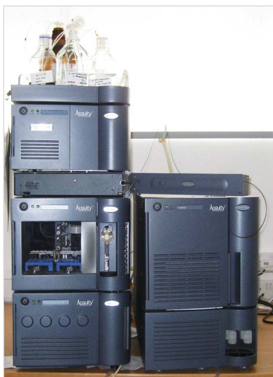
Picture 2.2 ACQUITY TQD UPLC-MS/MS system (Waters) used for the analytical determinations at UCY.
