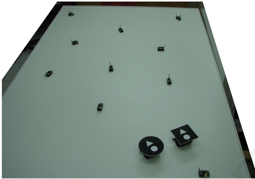
Figure 11.7: The experimental mixed WSN scenario setup consisting of twelve stationary and two mobile sensor nodes
