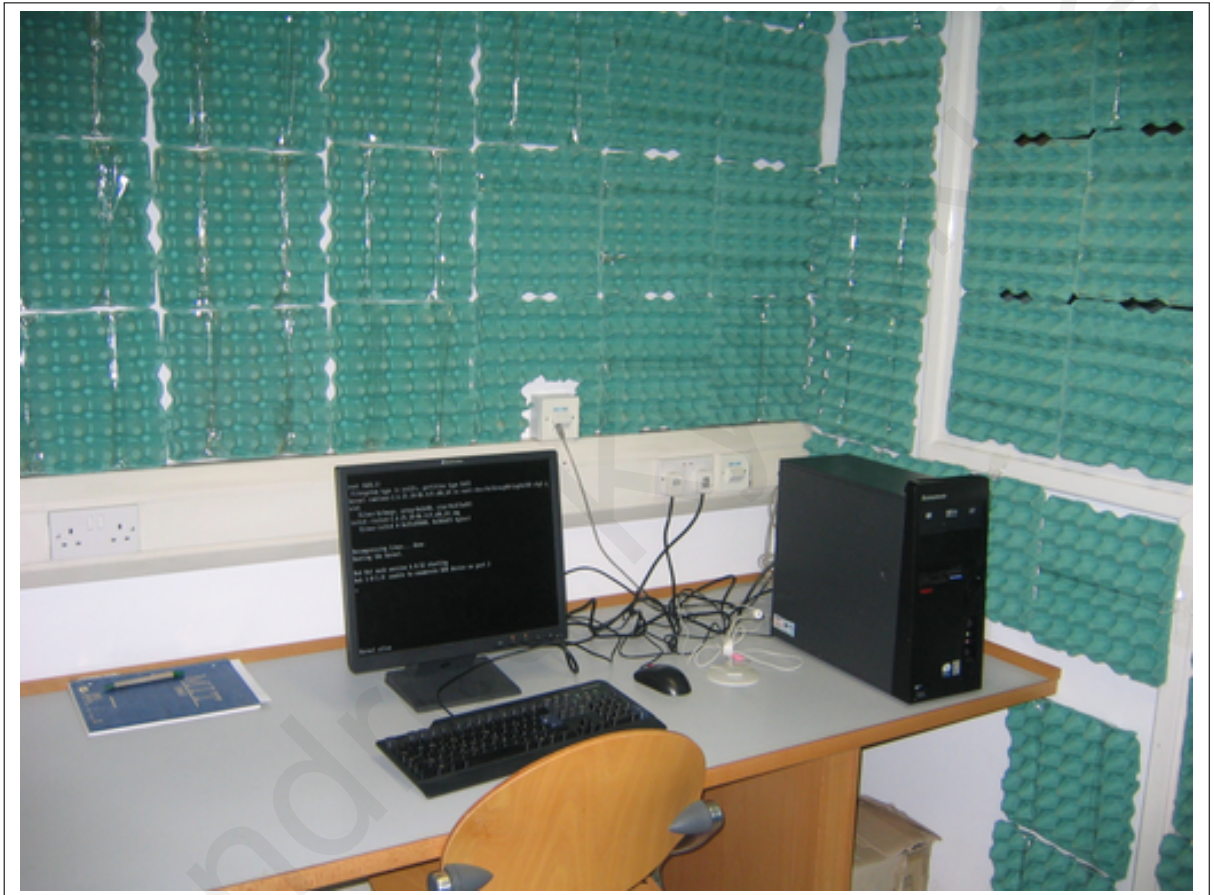
Figure 2.2: A photograph of the recording room showing the computer and microphone used for the recordings. The walls are covered with egg cartons to reduce reverberation.
