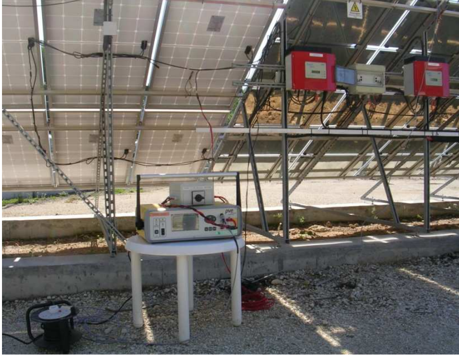
Figure 6.1. Outdoor temperature coefficient evaluation apparatus. The modules under investigation are first shaded and after the cover is removed, I - V curves are stored at different temperatures, using the connected PVPM1000.
