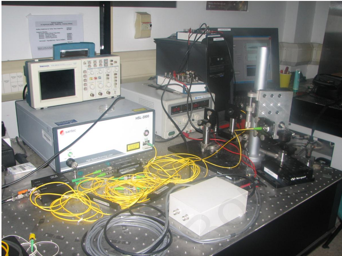
Figure 3.2 A photograph of the Swept Source OCT System
