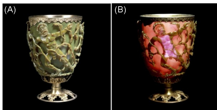
Figure 1.1: Photographs of the famous Lycurgus Cup which displays a different color depending on whether it is illuminated (A) externally, or (B) internally. For details, consult website of the British Museum [14], and Freestone et al. [15].
