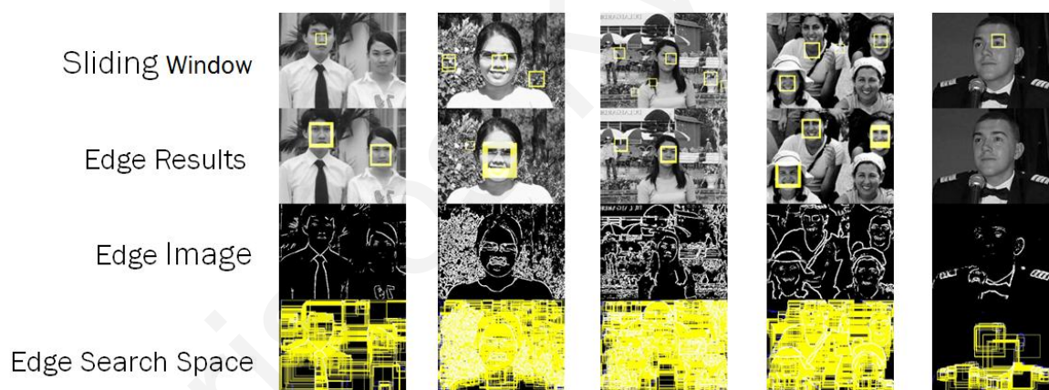
Figure A-3. Detection results using edge and compared to sliding window
