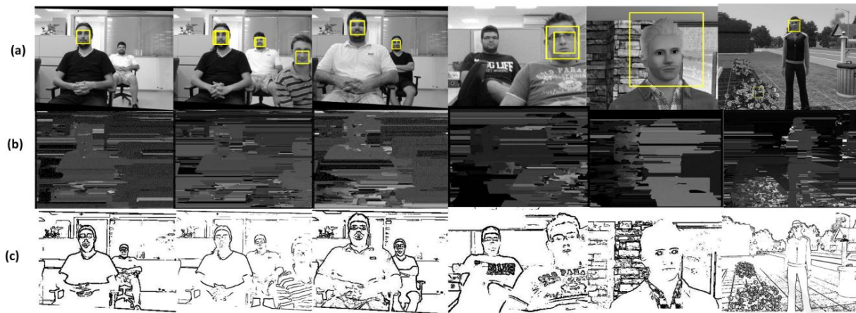
Figure 5-14. Depth and edge directed face detection results
