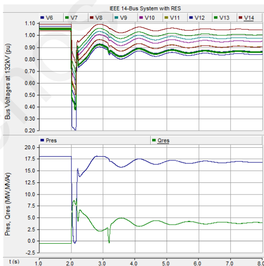
Fig. 7.4. IEEE 14-bus test system response when the RES operates according to the current grid regulations with k=2 .
