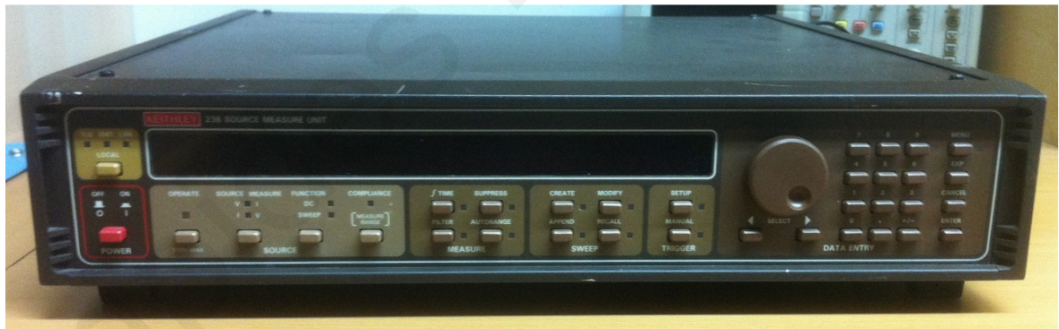
Figure B.7: The Keithley 236 SMU used for testing the neuromorphic chip.
