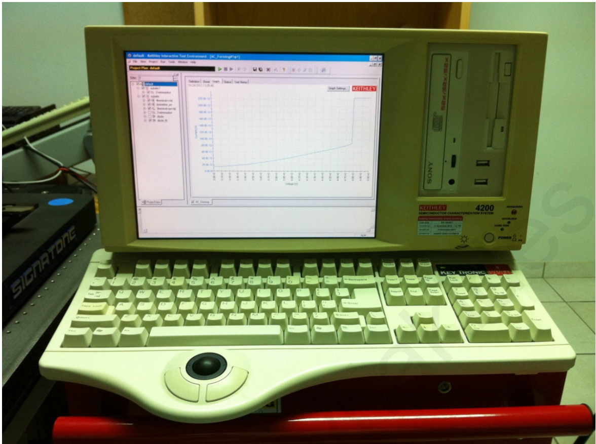
Figure B.2: Keithley 4200-SCS Parameter Analyzer for low-level measurements.
