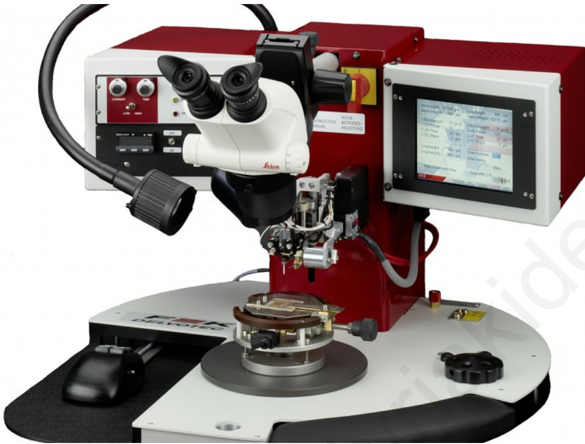
Figure B.8: The F & K Delvotec 53XX wirebonder used to connect the fabricated chips to a package.
