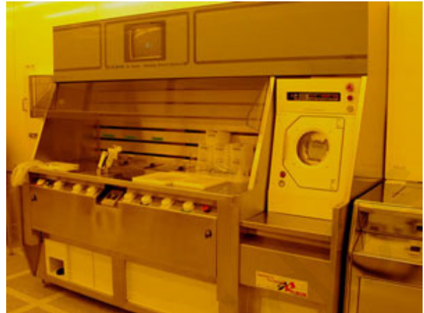
Figure A.8: Plade Solvent wet bench.
