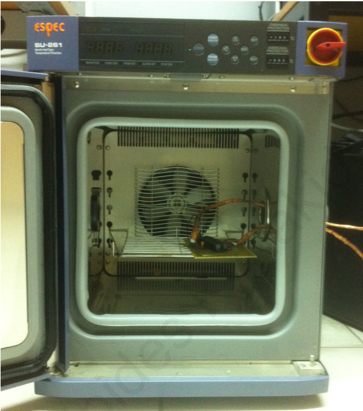
Figure B.1: The ESPEC SU-261 temperature chamber, shown with a sample loaded for testing, used for controlled heating of the NiTi devices.
