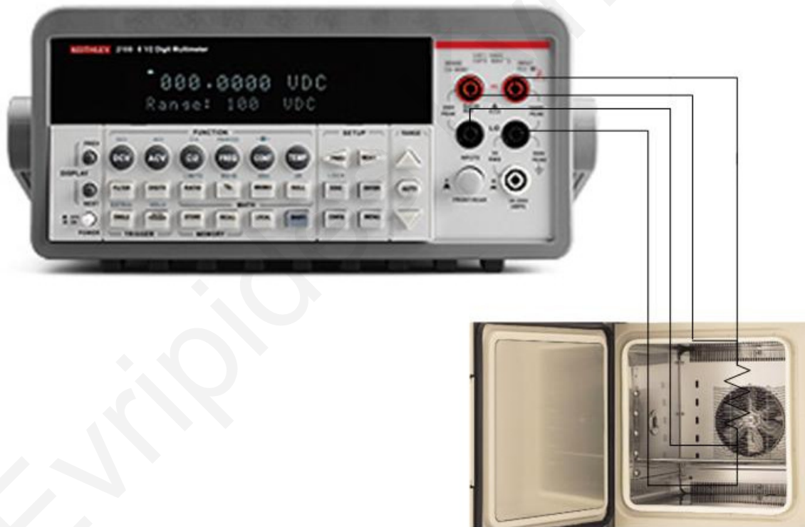
Figure 3.5: Four-wire resistivity measurements: The Keithley 2100 DMM, used to measure the NiTi device resistance during heating, connected to the ESPEC SU-261 temperature chamber, used for controlled heating of the NiTi devices.
