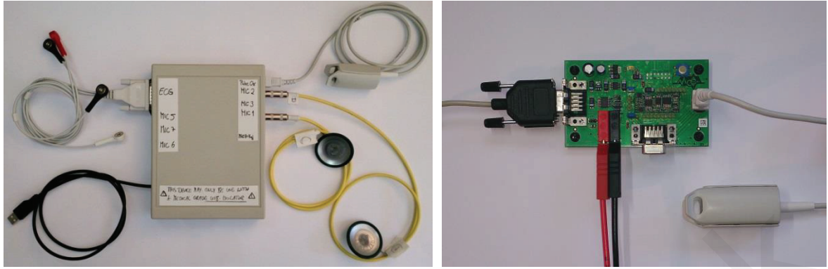
Figure 52: 1) Electronic parts embedded in a robust, shock, dust and splash water resistant housing; 2) Corscience's ChipOx development kit with interface to PC, power supply and finger sensor.
