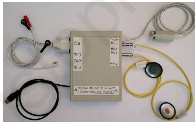
Figure 54: Electronic parts embedded in a robust, shock, dust and splash water resistant housing.
