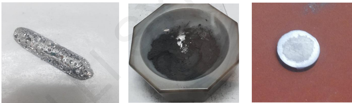
Figure 2.1. a) The obtained BST ingot for the melting, b) the agate mortar with the powder, c) the cold or hot press pellet.
