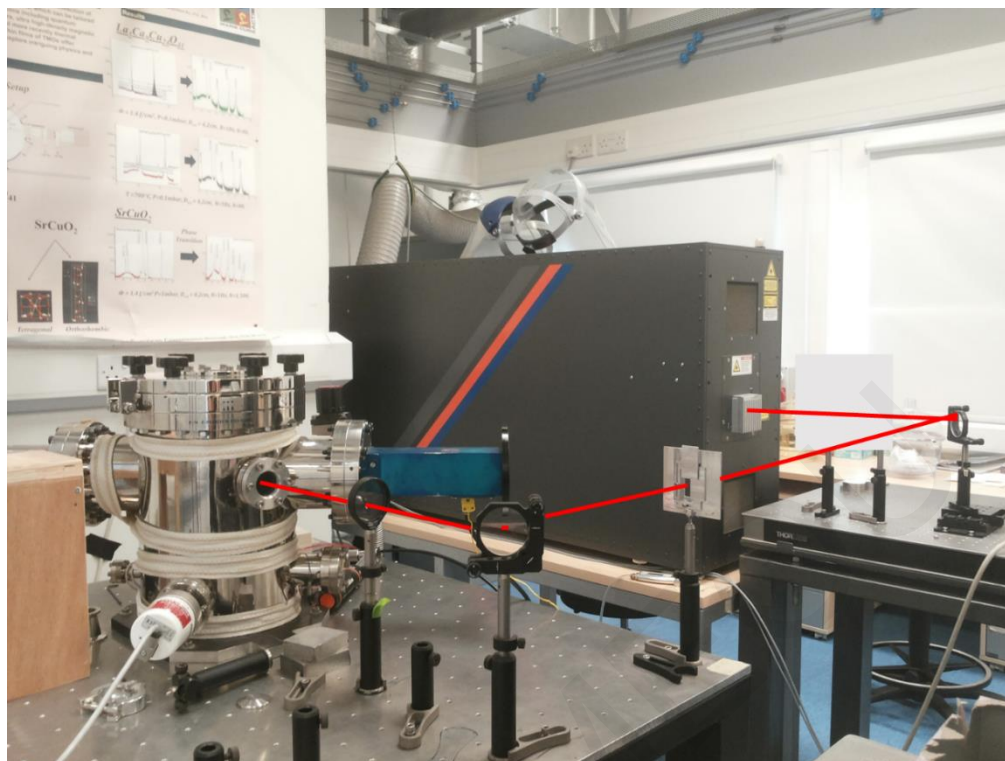
Figure 2.4. PLD system in our Lab. The red line presents the path of the laser beam to the chamber.
