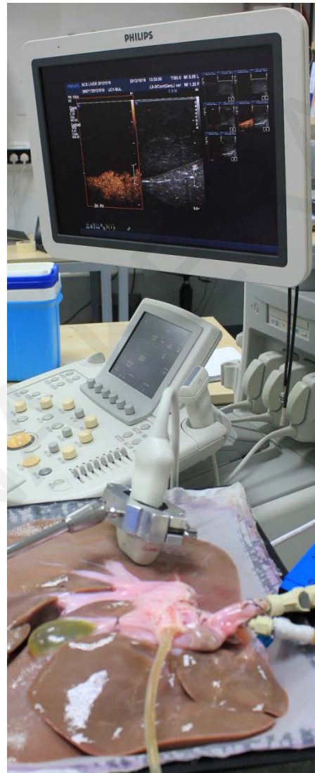
Figure 2.2: The iU22 ultrasound scanner (Philips Healthcare, Bothell, WA, USA) is positioned alongside the organ and 3 different probes are employed: (i) The L9-3 (shown here) acquires images from a fixed location over time, (ii) the L12-5 (not shown here) scans the entire organ to gauge percent perfusion over time, and (iii) the C5-1 (not shown here) is used to destroy bubbles between readings.
