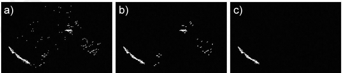
Figure 2-3: Extraction of the largest moving structure from the \{M_i\}_{i=1}^{\hat{N}} sequence: a) threshold image to binary by the 30% of the maximum pixel value, b) remove single pixels, and c) keep only the first largest structure.
