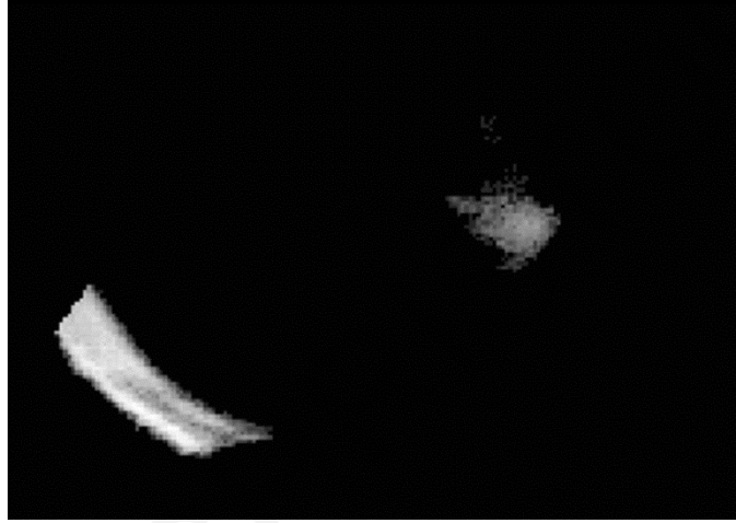
Figure 2-4: Example motion information matrix (MIM). Observe the two main areas in which motion occurs. The dominant structure producing motion is the diaphragm. Note that the values shown have been log-compressed to make the data easier to visualize.
