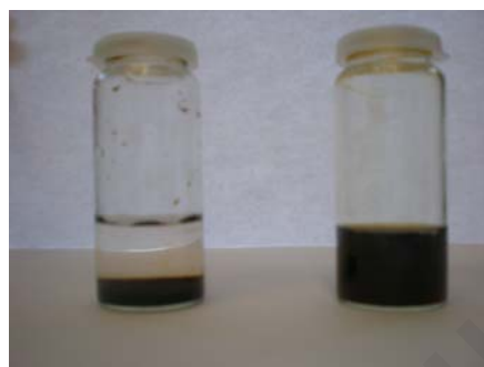
Figure 4.18. (a) Unstable solution of SWCNT/ \text{Fe}_x\text{O}_y system in the absence of the diblock copolymer, (b) Stable aqueous solution of the SWCNT/ \text{Fe}_x\text{O}_y /PEGMA 132 -b-AEMA 42 .
