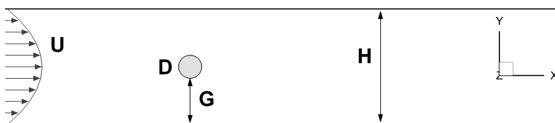
Figure 2.7: Geometrical configuration for the case of a circular cylinder confined in a plane channel.
