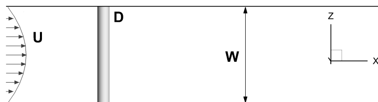
Figure 2.10: Geometrical configuration for the case of a circular cylinder confined by end plates.
