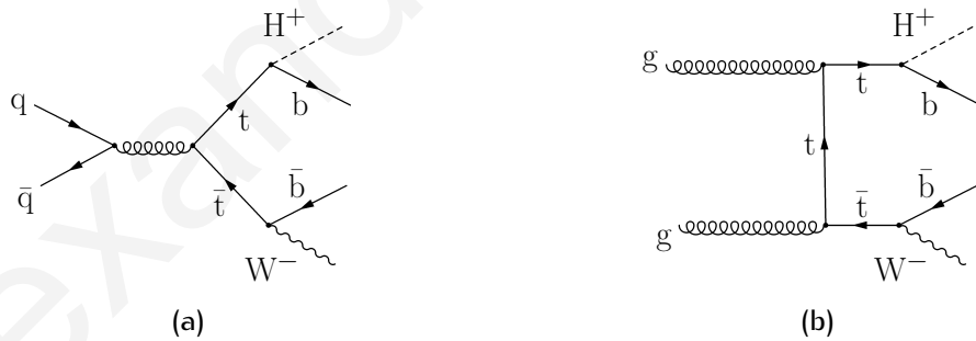
Figure 2.6: Typical Feynman diagrams for the light charged MSSM Higgs boson production at the LHC.
