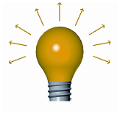
Figure 9: The radiant power \Phi of a light source is given by its total emitted radiation.
