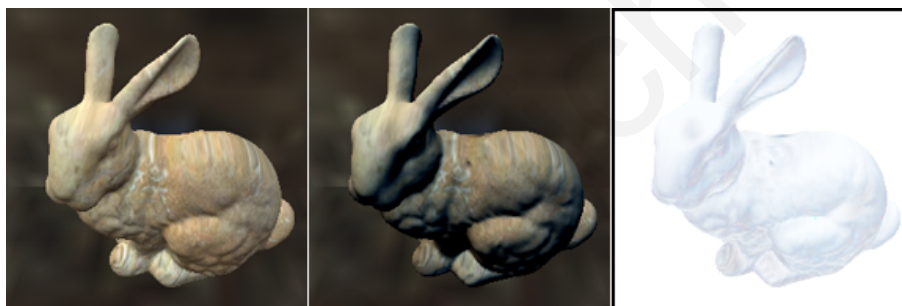
Figure 24: Self-shadows are also computed at run-time using precomputed FIVs. Only direct illumination without considering self-occlusions (left), direct illumination and self-shadows (middle), isolated self-shadow (right).
