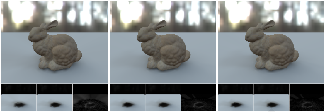
Figure 18: The bunny at different sampling rates ( \vartheta, \varphi, \varrho ): Samples = (32,17,15) (NRMSE = 0.023) (left), Samples = (64,33,30) (NRMSE = 0.008) (middle), Samples = (256,129,30) (NRMSE = 0.007) (right). The small images show the shadow only of the result of the proposed technique (left), the ground truth shadow (middle) and the difference of the two (right).
