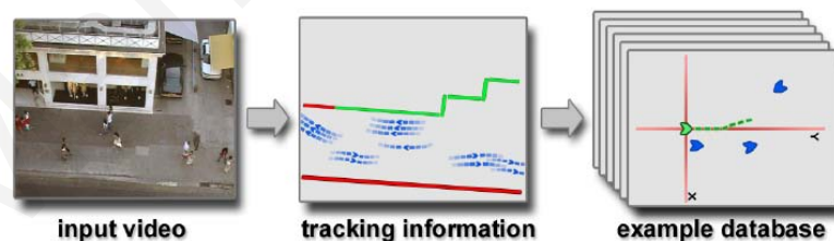
Figure 2: Pre-process phase: the input video is manually tracked generating a set of trajectories. These are encoded as examples and stored in the trajectory database [6].
