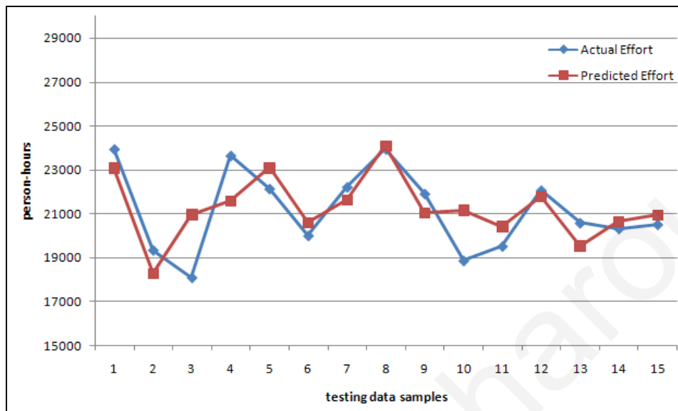
Figure 4.8: Partial data samples of Actual vs. Predicted Effort during validation (testing) experiments for the Desharnais dataset using a 3-8-1 ANN topology
