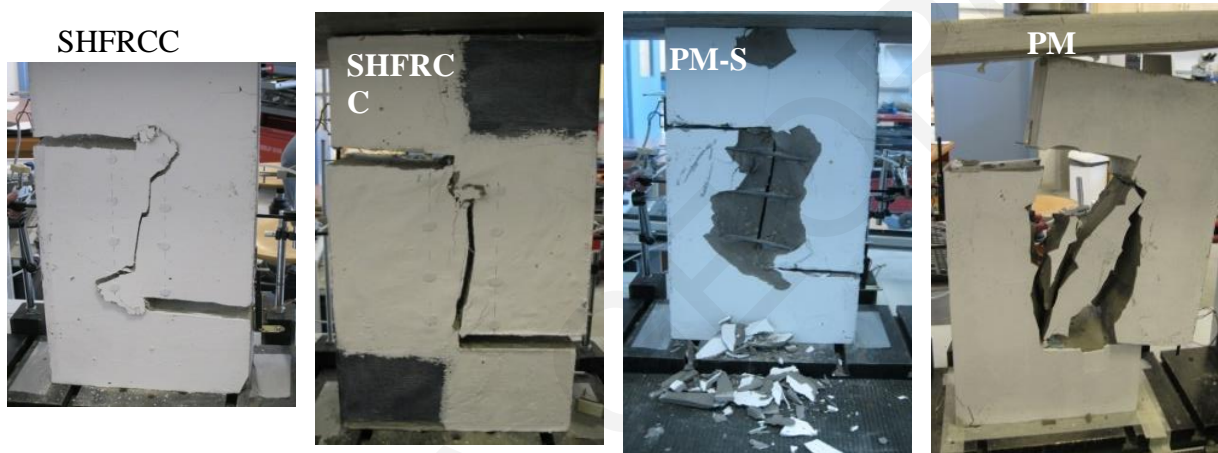
Figure 8.2: Push-off crack patterns for all specimens
