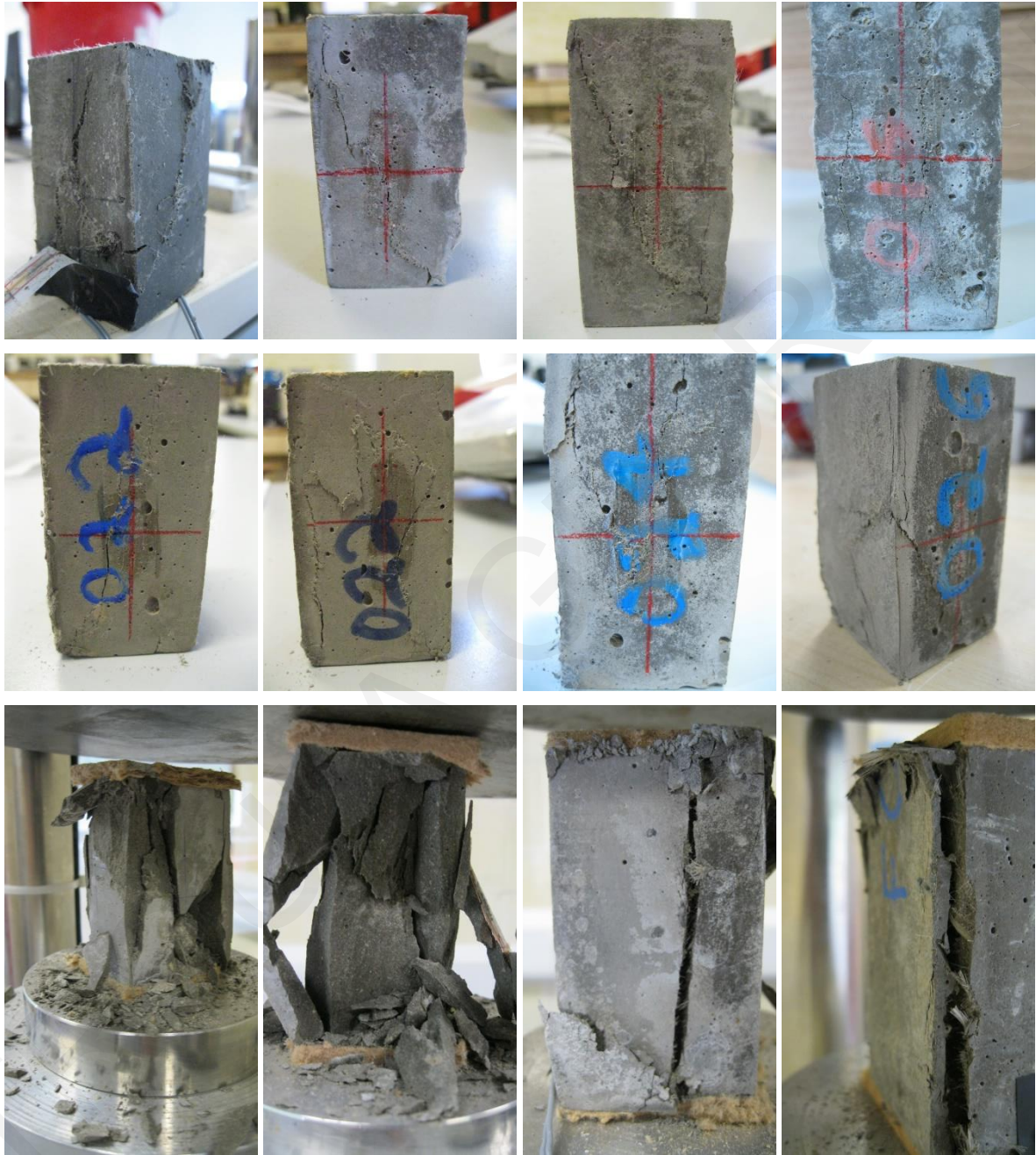
Figure 3.8: Compressive prism specimens failure cracks (O11, O12, O13, O16, O22A, O22B, O24, O26, NCC1, NCC2, FCC1, FCC2)
