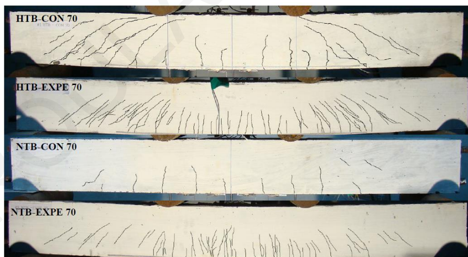
Figure 7.1: Failure behavior of beams (130×170×1460 mm) [138]
