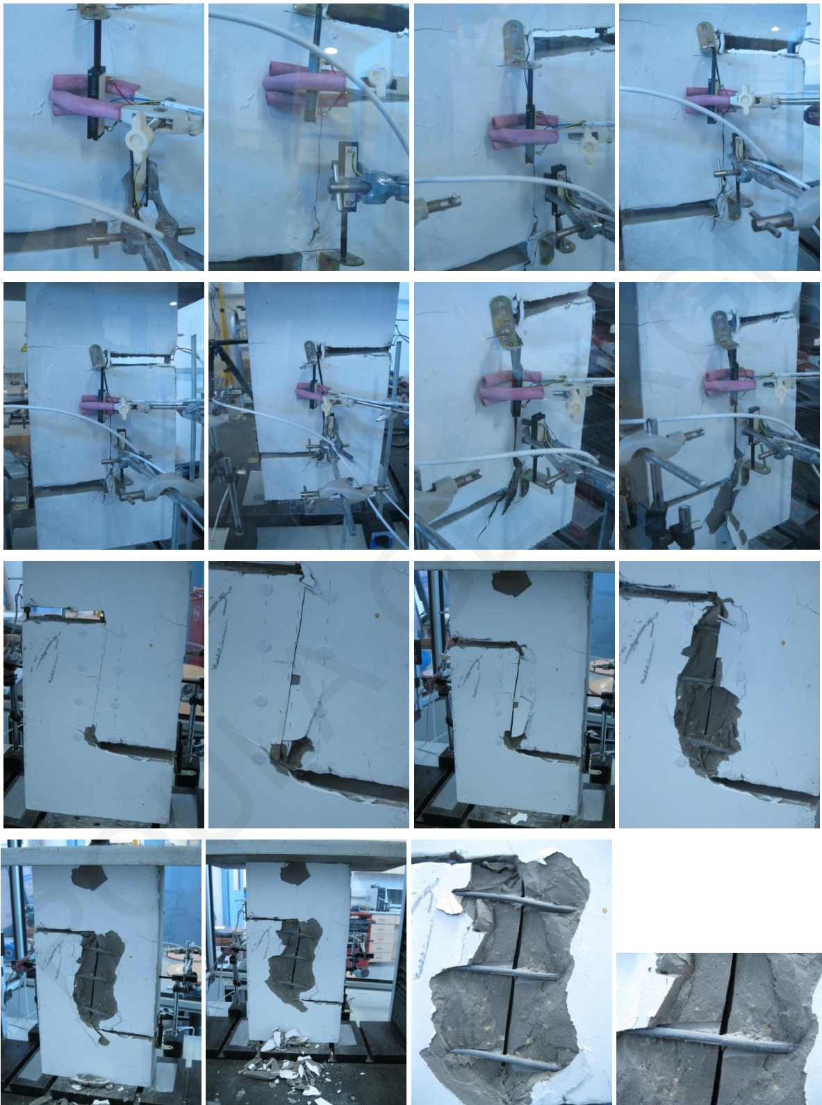
Figure 8.3: Crack sequence on both sides of a specimen without fiber but with steel reinforcement crossing the shear plane (Specimen F5-S1 or PM-S)
