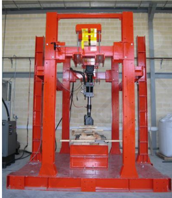
Figure 10.14: MTS hydraulic actuator attached on a self-reacting steel frame
