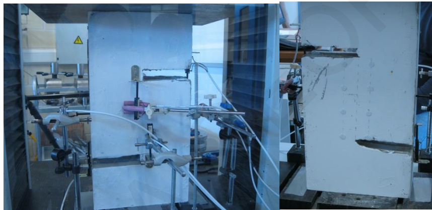
Figure 8.1: (a) Push-off specimen and dimensions, (b) LVDTs positions and measuring lengths, (c) steel reinforcement, d) definition of deformation for graphic presentation
