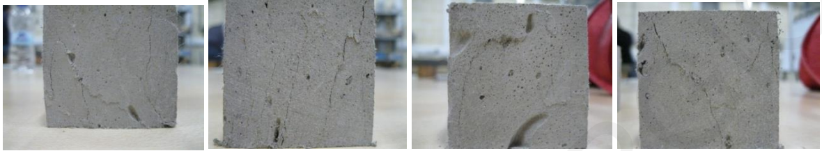
Figure 3.7: PP1B compression tests-failure cracks
