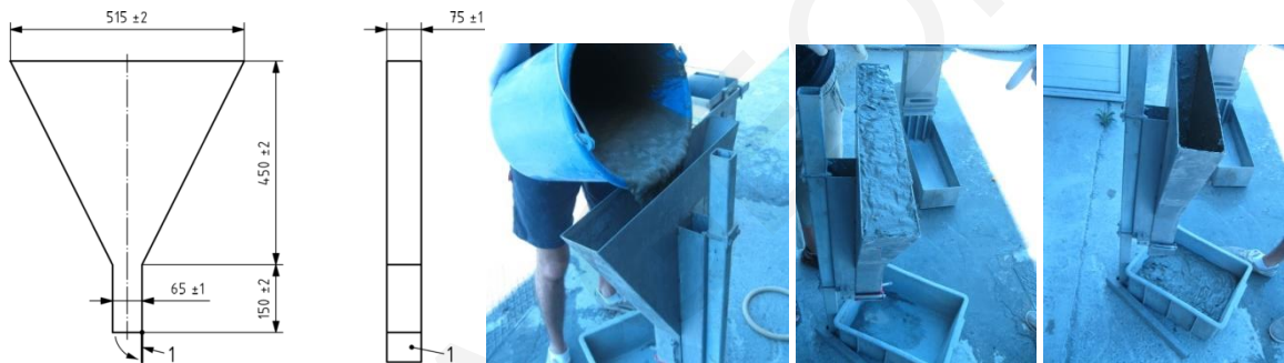
Figure 4.19: V-funnel test equipment (dimensions in mm)
