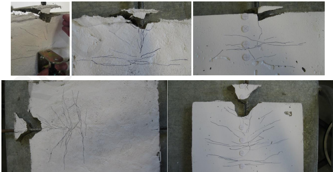
Figure 9.21: Cone shape failures of specimens F8A5C11 (top) and F8A12C11 (bottom)
