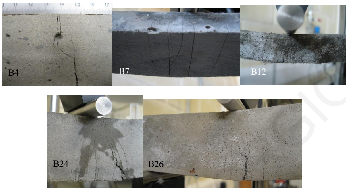
Figure 3.19: Crack behavior of various fractions and types of coating at 28 days
