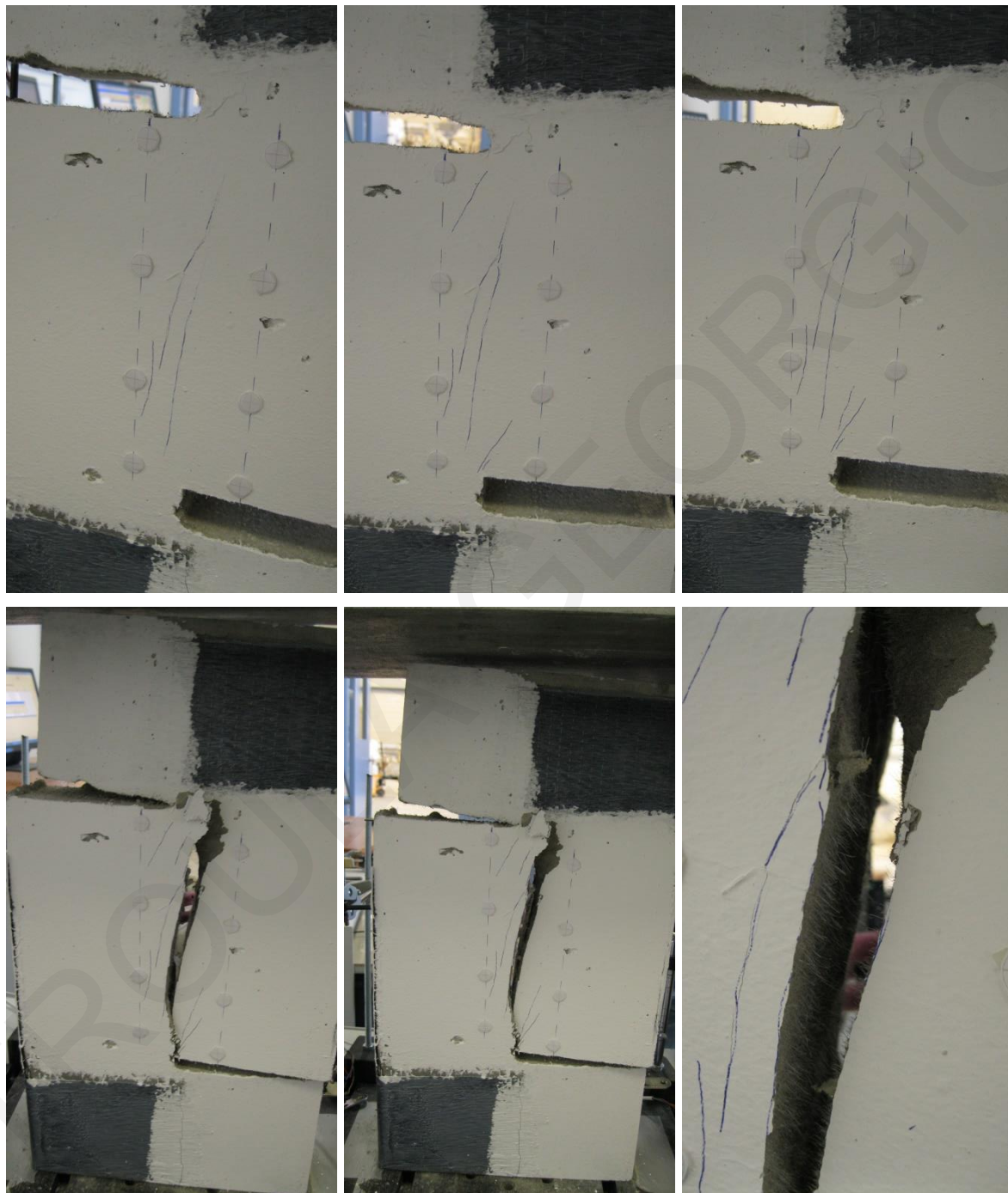
Figure 8.4: Crack sequence on both sides of a specimen without fiber but with steel reinforcement crossing the shear plane (Specimen shF7-1 or SHFRCC)
