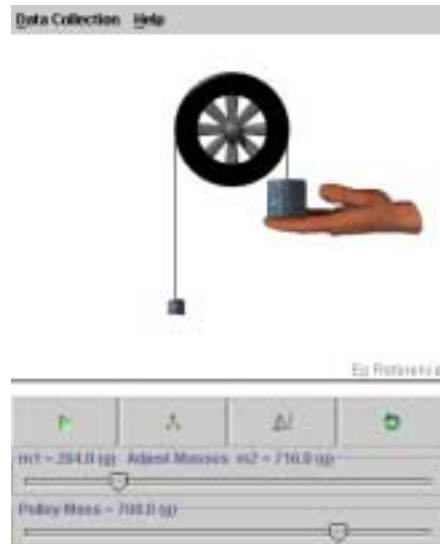
Figure 6 The applet atwood which simulates the motion of an Atwood’s pulley. By pressing the appropriate buttons the student can display free-body forces or a graphical representation of salient variables.
