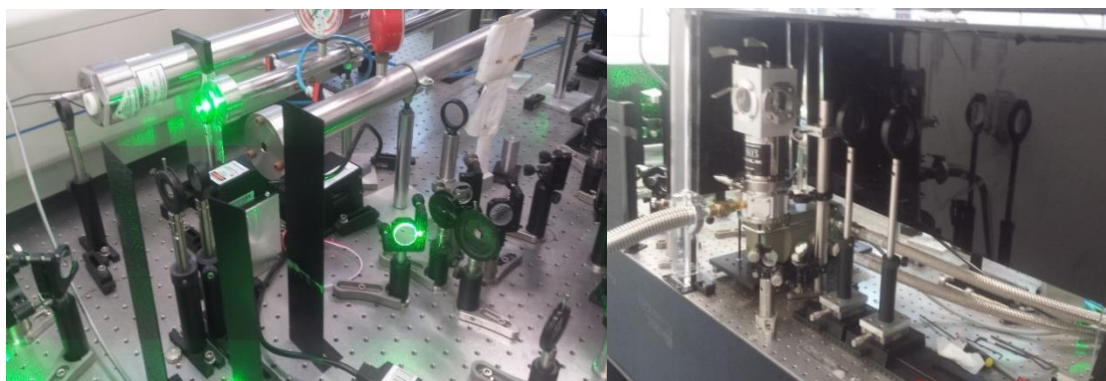
Figure 3-4 Experimental setup for Resonance Raman. Left: light at 532 nm coming out from the Raman shifter and properly conveyed through the optical system towards the sample (right). Right: sample holder (placed inside a closed-cycle cryostat system), collecting and collimating lenses.
