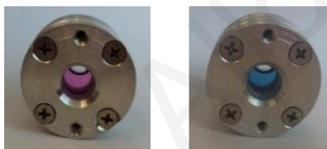
Figure 3-6 Image of the custom cryocell with aqueous MEG-PBI solutions at RT (left) and 313 K (right).
