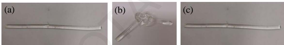
Figure 3.4.6. Shape memory effect for the water-swollen (DMAAm 80 - co -DDAAm 20 )- co -HDDA 1 randomly cross-linked copolymer network. (a) Initial shape at 25 °C, (b) fixed knot shape after heating the gel up to 50 °C and cooling down to 25 °C, (c) recovered shape after heating the gel up to 50 °C.
